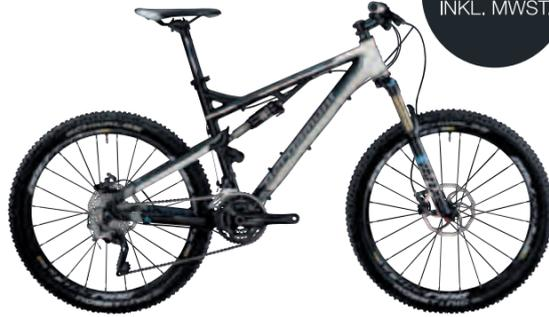
Tapered Headtube - Fox 32 Float 26" CTD O/C, Evolution-Series 120 mm Fork - RockShox Monarch RL Shock - Shimano Deore XT 3x10-Speed Drivetrain - Avid Elixir 5 hydraulic Discbrake - Mavic Crossride Disc Wheelset
